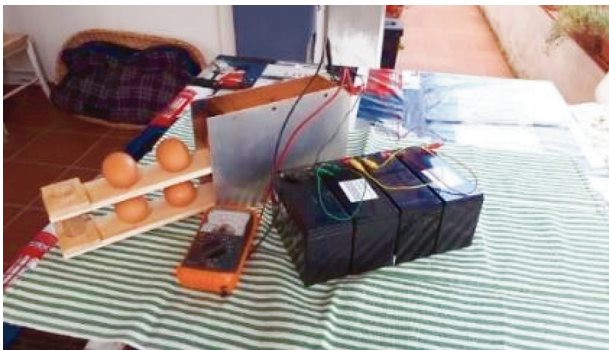
Device A. Note the condenser, 4 batteries 12/V in series and the voltmeter
